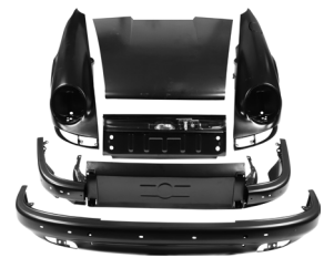
Backdate kit 911 F Body, heavy modifications are required
