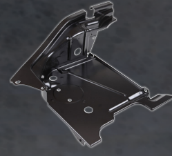
Engine cover, right. RS design // Dansk no. 591091-6 JP no. 1682602280 // OE ref. 964 106 283 76 Fits: Porsche 964 RS (3.6) 06/91-09/93
